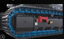
Reinforced lowerframe and undercarriage components
