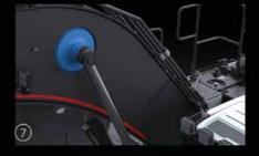
Reinforced boom cylinder cast bearing
