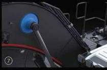
Reinforced boom cylinder cast bearing
