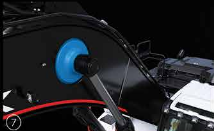
⑦ Reinforced boom cylinder cast bearing
