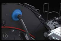
Reinforced boom cylinder cast bearing
