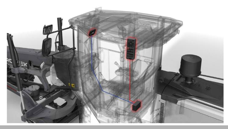
Hidromek Opera is an interface that facilitates communication between the operator and the machine. Operator may easily switch between menus in Opera, and check the status of the machine, and change the settings.
